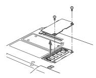
Figure 4-9 Opening the Memory Upgrade Compartment
